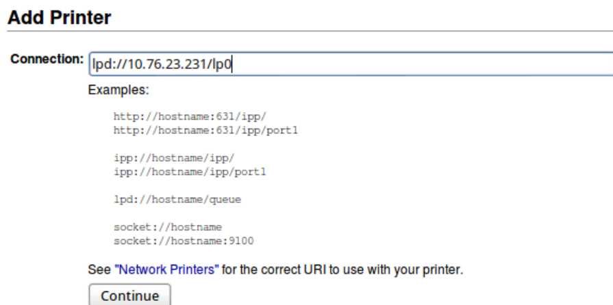
Figure 3.5: Local USB printers can easily be shared: This screenshot shows adding USB printer /dev/usb/lp0 on LessLinux host 10.76.23.231 to a CUPS server that centralizes spooling.
